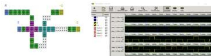
Figure 13 Layout of SR Latch and its waveform
